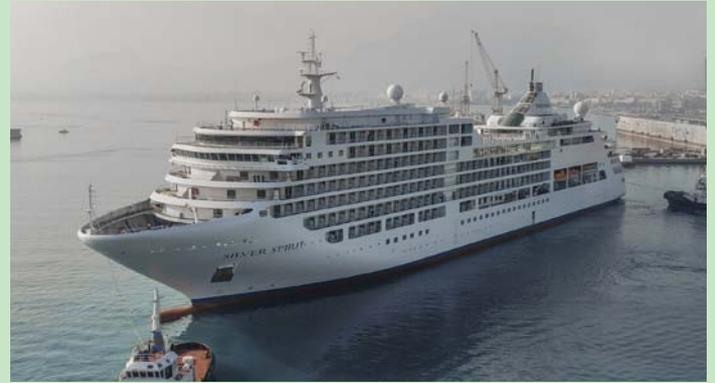
**SILVERSEA'S** *Silver Spirit* has emerged from drydock 15m longer following completion of a complex lengthening and refurbishment project.
