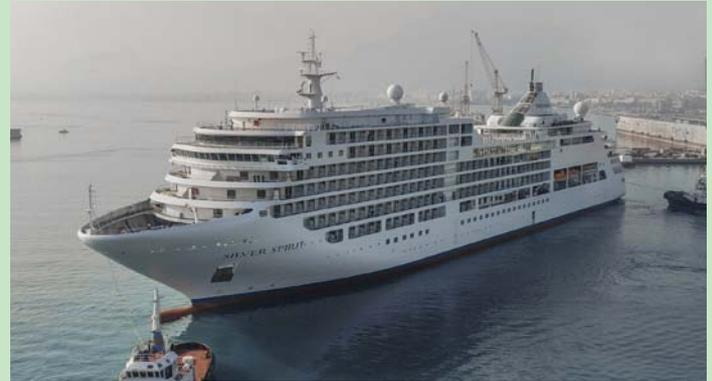
**SILVERSEA'S** *Silver Spirit* has emerged from drydock 15m longer following completion of a complex lengthening and refurbishment project.
