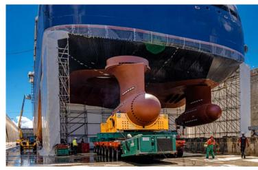
THE final stages in the construction of Ponant's Le Commandant-Charcot have begun, with the ship arriving in Saint-Nazaire to be fitted with Azipod propulsion systems.
