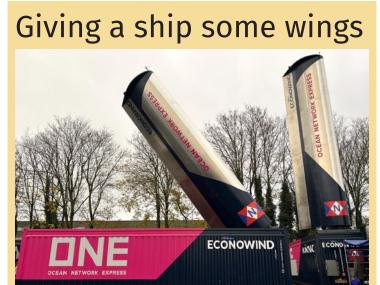
**DUTCH** maritime windpowered technology specialist Econowind has confirmed a collaboration with Singaporebased Ocean Network Express (ONE) to install two "containerised wind assist devices" on a ship carrying cargo across the Pacific.
